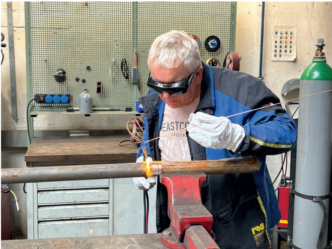
▲ Pic 2. A metal welder preparing a lance for a future job.
